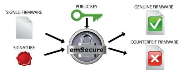
On a firmware update and when starting the product, the bootloader will verify the firmware by its signature. If they match, the firmware is started, otherwise the application will stay in the bootloader or even erase the firmware.
