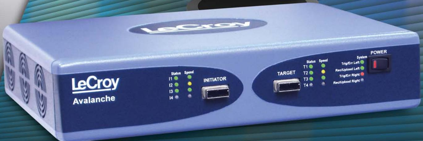
**LeCroy, a worldwide leader in serial data test solutions, creates advanced instruments that drive product innovation by quickly measuring, analyzing, and verifying complex electronic signals. The Avalanche SAS and SATA Protocol Analyzers are LeCroy's newest systems that decode data rates up to 6Gb/s Serial Attached SCSI (SAS) and 6Gb/s Serial ATA (SATA) traffic.**
