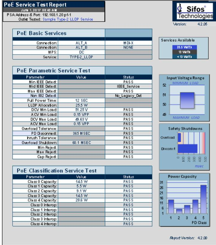
The report provides three tabular tables that include results from **PoE Basic Services**, **PoE Parametric Service** testing, and **PoE Classification Service** analysis.
