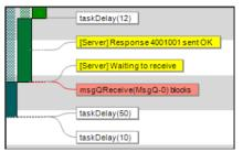
Tracealyzer features **User Events**, allowing you to log any event or data in your application. User Events appear as yellow labels in the trace view and can be used as an alternative (or complement) to classic debug "printf" calls and for plotting of logged data. Since User Events are stored very quickly, they can be used also in time-critical code. Moreover, they are shown in the trace views so it is easy to correlate them with overall system behavior.
