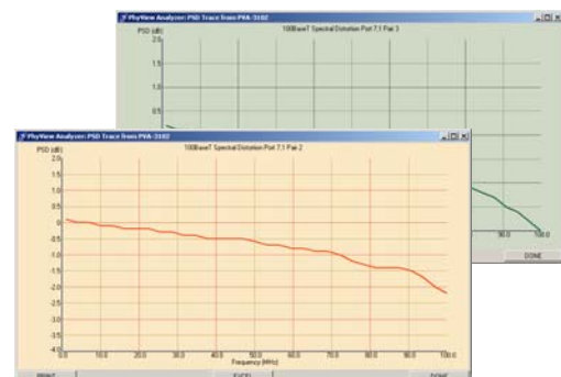
PSD on Pairs 2 & 3 at 100BaseT
