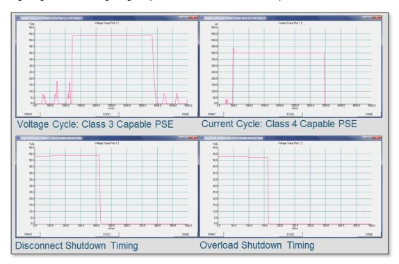
Two additional waveforms available are Disconnect Shutdown and Overload Shutdown. These waveforms may utilized to visualize the PD service outlet response to either a PD disconnect or a PD transient overload condition. Both conditions should result in power removal in order to prevent damage to network devices when plugged into
